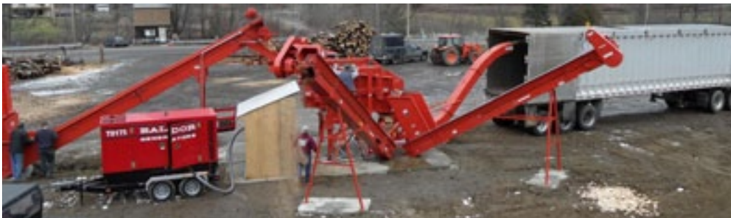
A woodchip screener used to remove over-sized woodchips and fine dust from the bole chips before they are loaded into a trailer for delivery to a woodchip heated facility.
