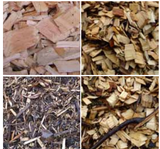
Woodchip quality grades, from top left clockwise: clean or paper-grade; bole; whole-tree; and urban-derived.
