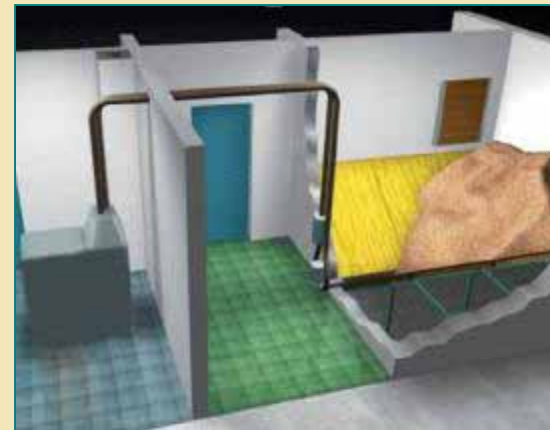
V bottom rigid bin in storage room
