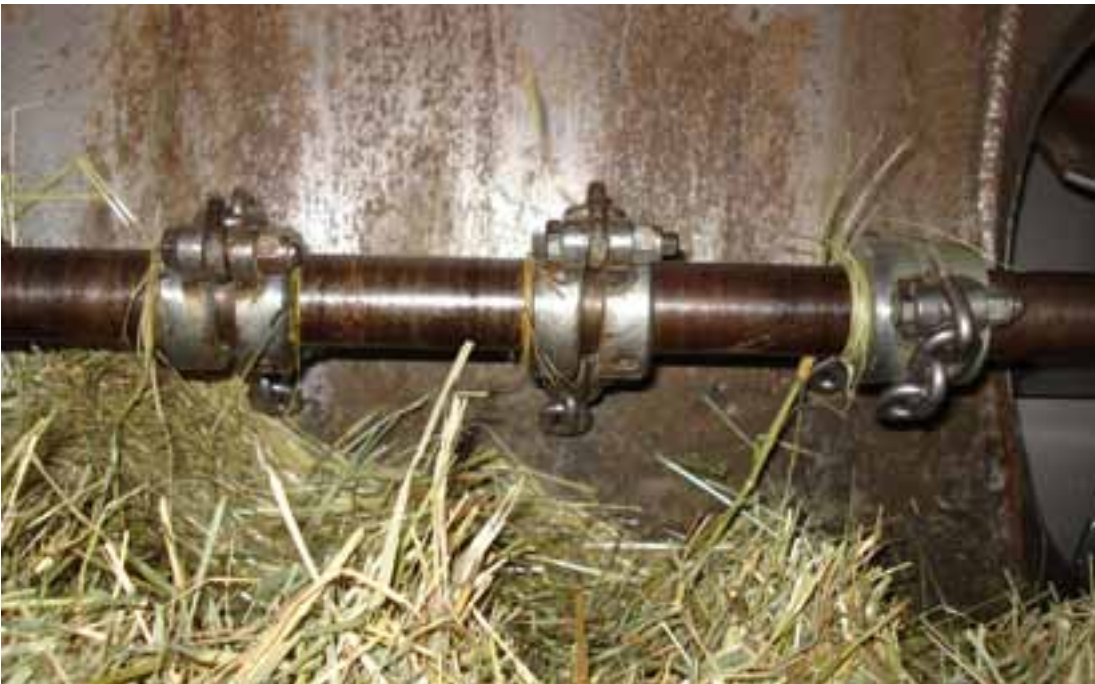
From top clockwise: inside of the hay bale mulcher/blower unit; a tractor-mounted, PTO-driven hammermill was used to re-grind grass fibers prior to pelletization; grass after using the bale mulcher and hammermill.
